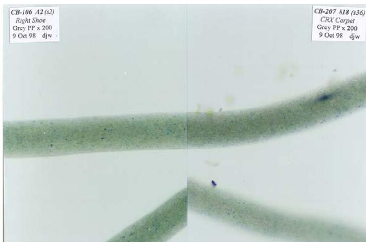
**Figure 5:** Comparison microscopy of a grey polypropylene from the shoes (left) and the Honda CRX carpet (right)
