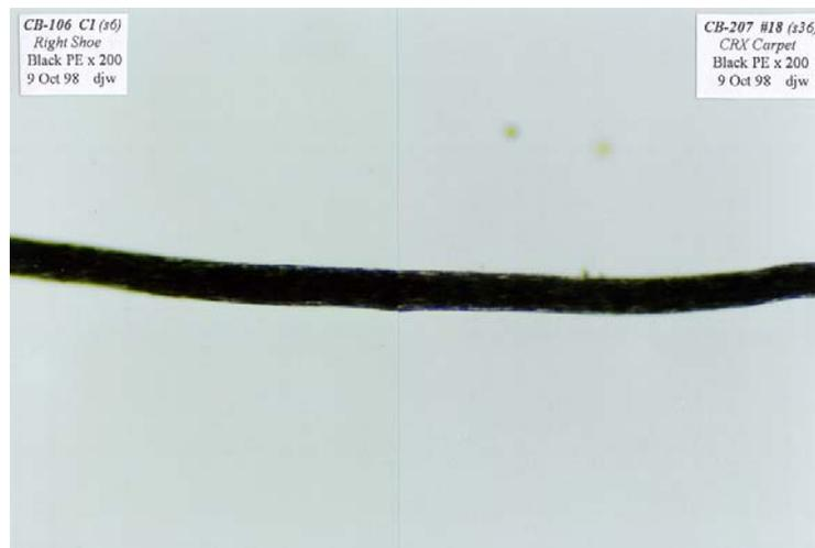
**Figure 3:** Comparison microscopy of a black polyester from the shoes (left) and the Honda CRX carpet (right)
