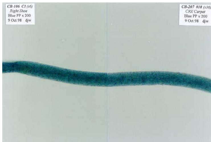
**Figure 4:** Comparison microscopy of a blue polypropylene from the shoes (left) and the Honda CRX carpet (right)
